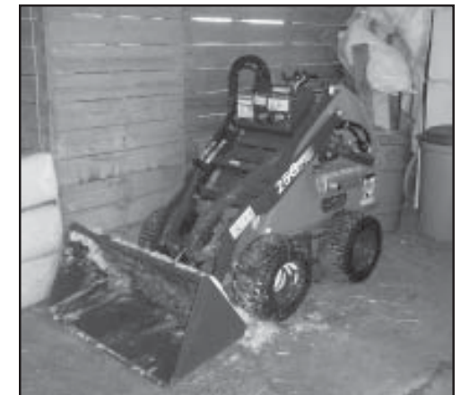
DVR purchased a small skid steer to aid Peterson in cleaning stalls and hauling manure, which was previously performed with a wheelbarrow, pitchfork and shovels.
