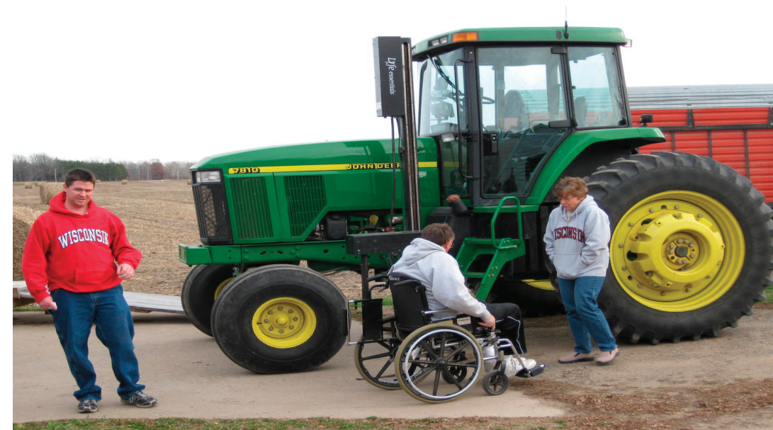
Jeff Kratochwill describes the lift features, while Larry Kuhl demonstrates the Life Essentials lift on his John Deere tractor and Larry's wife, Patty, watches Larry make the transfer.
