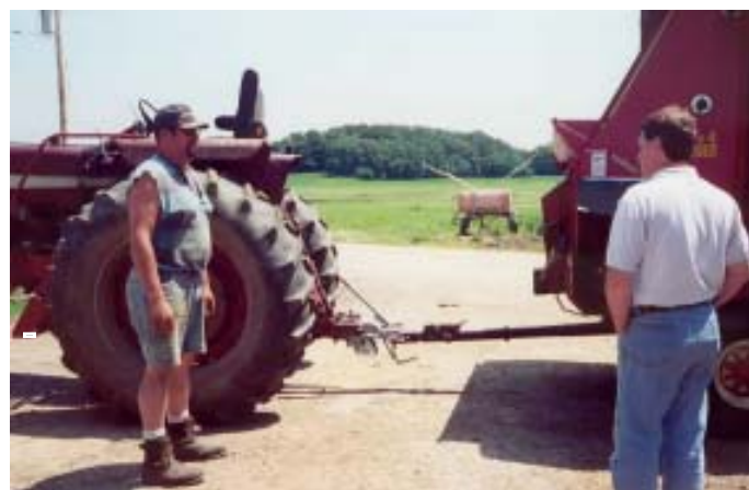
Marvin's son, Charlie, and Paul Leverenz stand next to a tractor fitted with extra steps and handholds, an air ride seat, and an Agri-Speed hitch.
