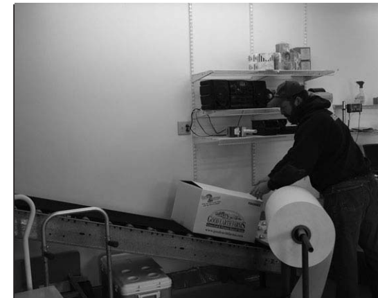
Modifications to the shipping room were made, by adding a conveyor belt to lift the boxes straight from the shipping table up and outside to the loading dock.
