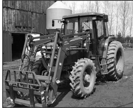
Unlike the old Leyland, the John Deere 6405 has an enclosed cab and an air ride seat.
