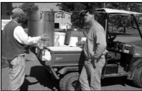
Purvis explains how an old water heater he mounted to the Kawasaki mule DVR provided makes for easy hauling of water and milk replacer to the calf hutches.
