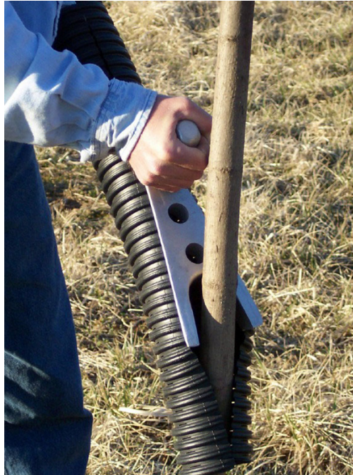
The tree guard zipper saves time, prevents hand strain.
